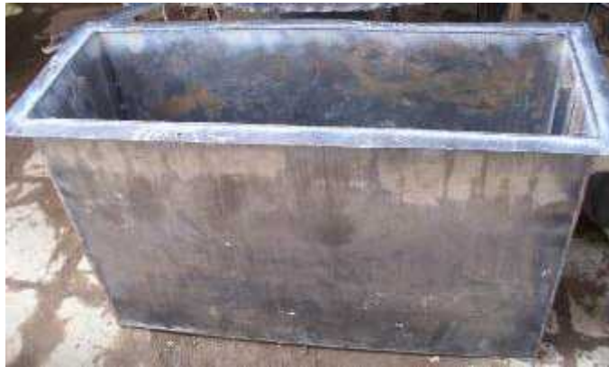
Picture 36: Flange welded onto the baking chamber
