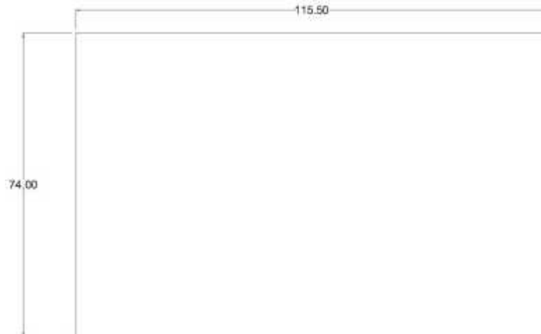
Figure 57: Dimensions of bottom piece for baking chamber
