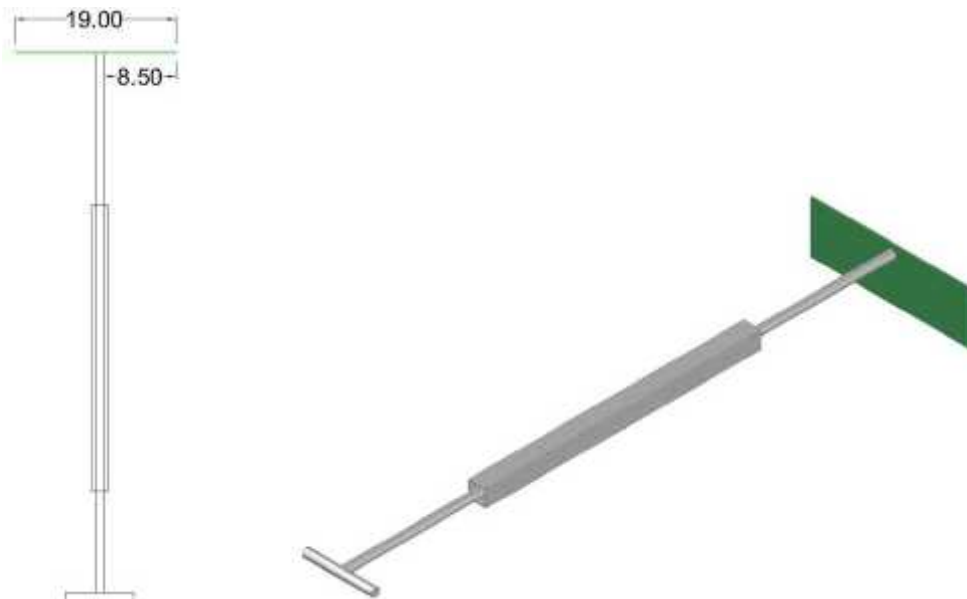
Figure 141: Dimensions for placement of scraper (left) 3D image of scraper assembly (right)
