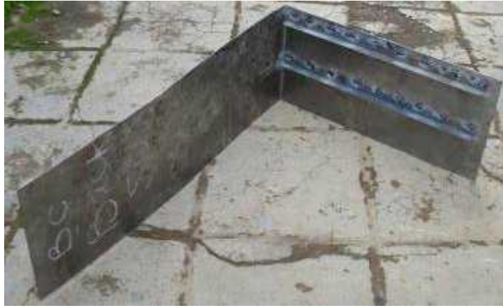
Picture 32: Image of angle bar rack supports attached
