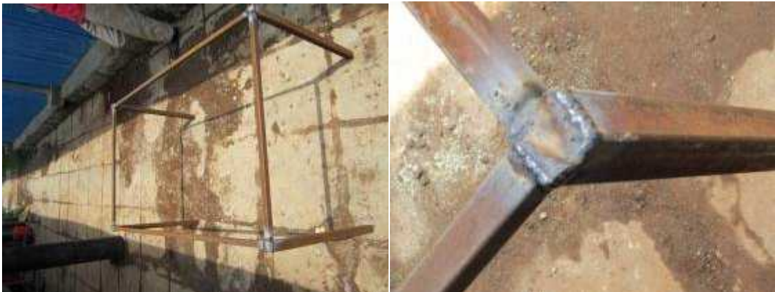
Picture 5: image of feet attached (left) close-up view of feet attached (right)
