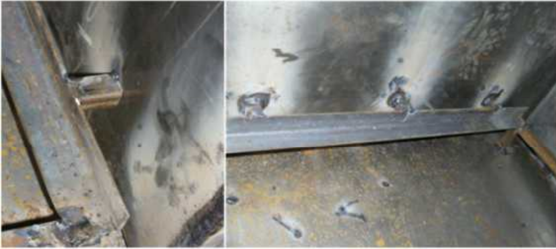
Picture 60: Close-up image of supports attached (left) image of supports attached as relates to entire oven
