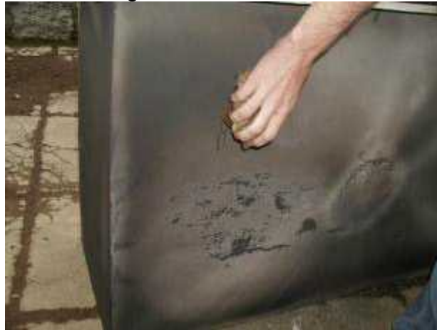
Picture 91: Image of cleaning outer surface of baking chamber
