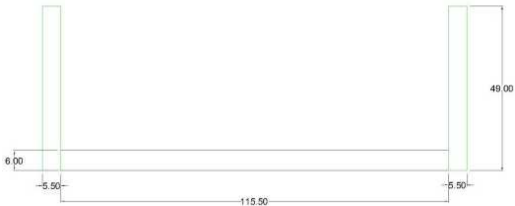
Figure 36: Dimensions for sides of the baking chamber flange attached to the bottom
