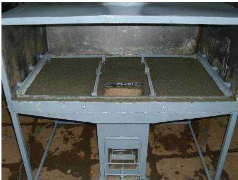
Picture 85: Pumice/concrete layer added to the taper
