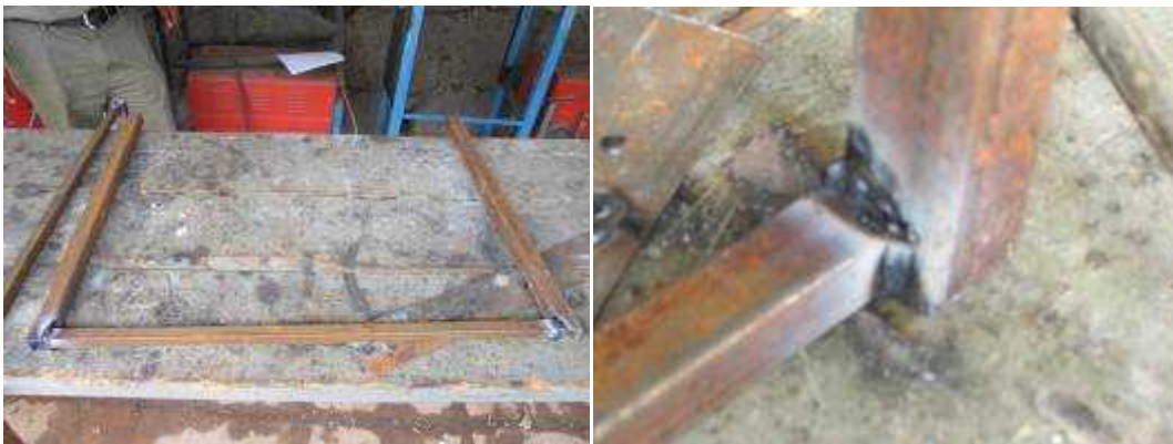
Picture 1: Image of U-shape (left) and image of 2x2cm square pipe flush with 3x3cm square pipe (right)
