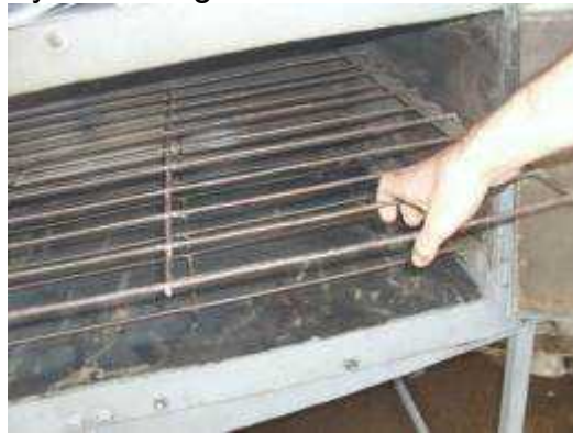
Picture 88: Image of rack removal
