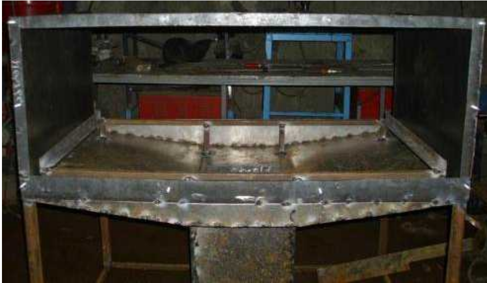
Picture 53: Image of oven chamber lip attached
