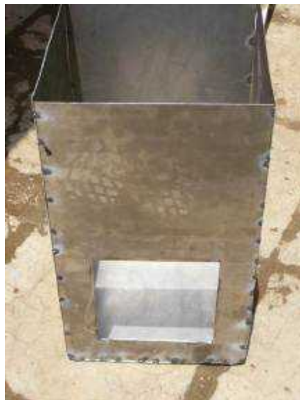
Picture 10: Completed metal combustion chamber
