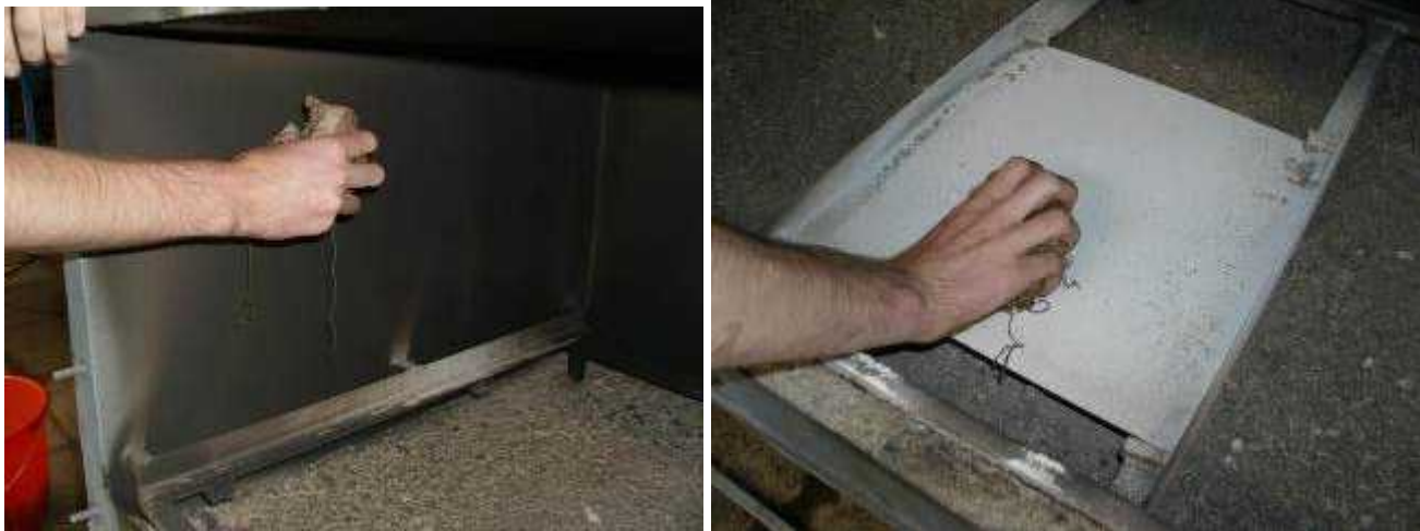
Picture 90: Image of cleaning oven chamber wall (left) and baffle (right)
