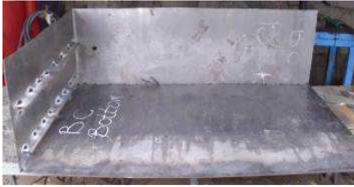
Picture 34: Image of bottom attached to the back/side of baking chamber
