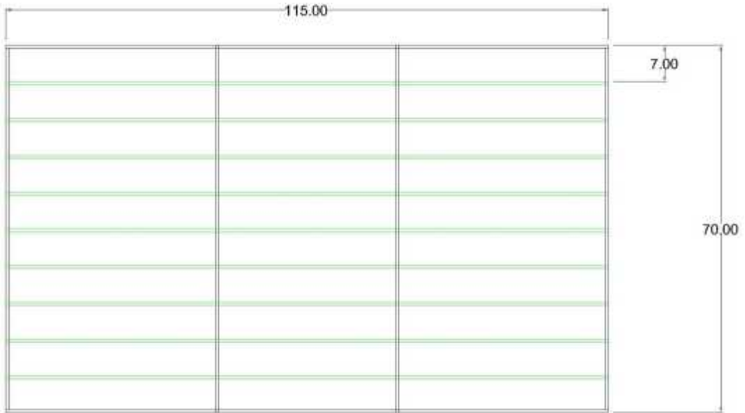
Figure 66: Dimensions for 9 pieces of 115cm round bar
