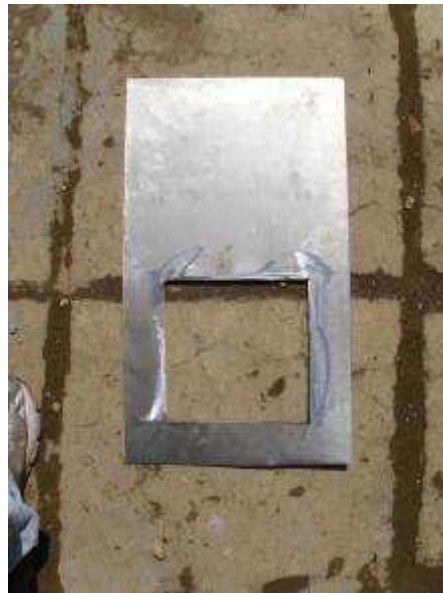
Picture 8: Image of cut combustion chamber face plate
