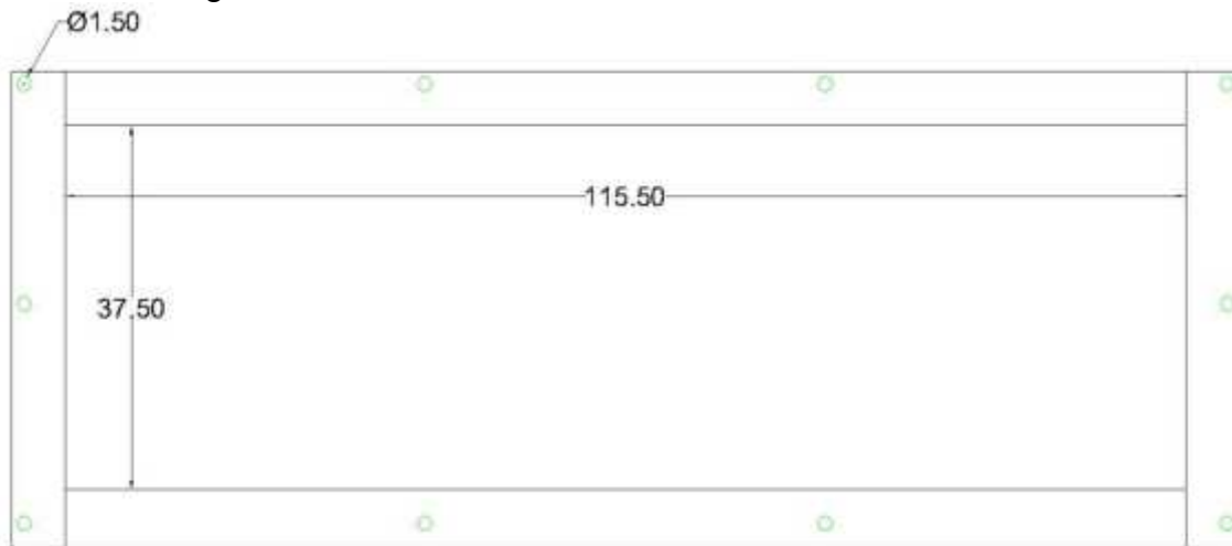
Figure 47: Dimensions for baking chamber flange bolt holes
