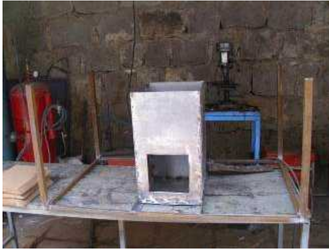
Picture 11: Image of combustion chamber added to base
