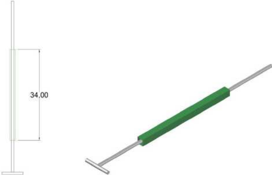
Figure 139: Dimension for square pipe (left) 3D image of round bar in square pipe (right)
