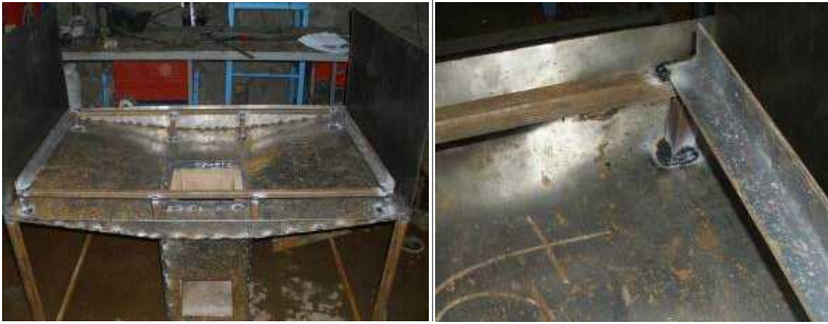
Picture 52: Image of attached outer supports (left) and close up of outer support on frame (right)
