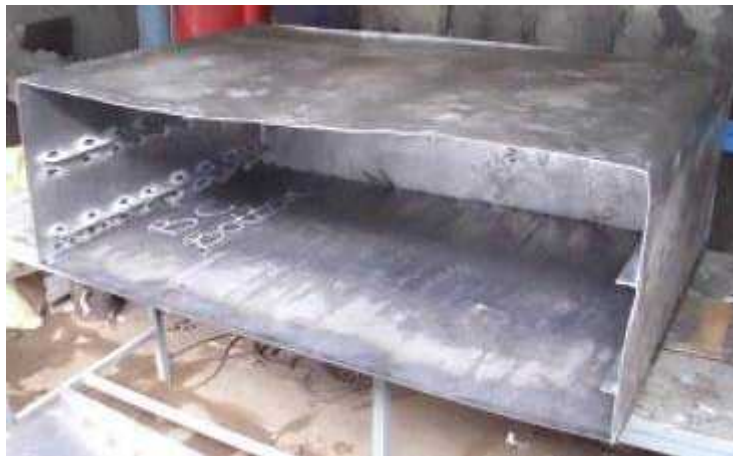
Picture 35: Image of top/side welded onto the baking chamber
