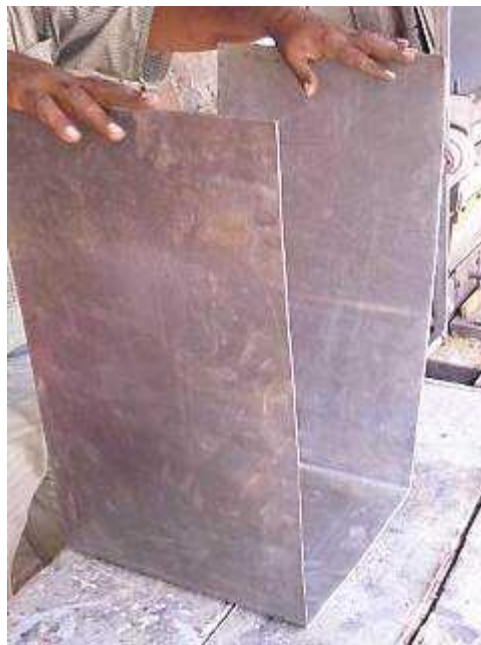
Picture 7: Folded sides and bottom of combustion chamber
