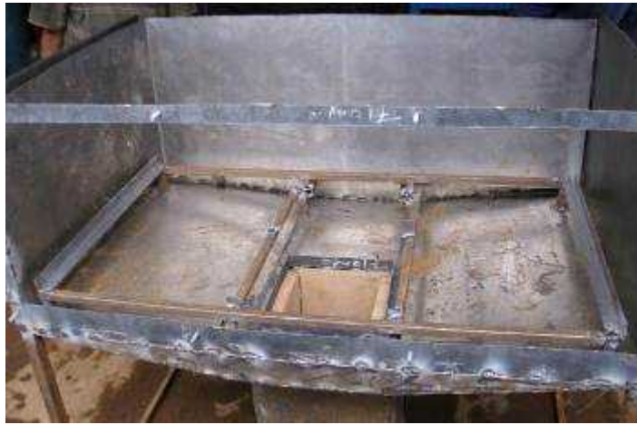
Picture 58: Image of side/back piece of barrier attached
