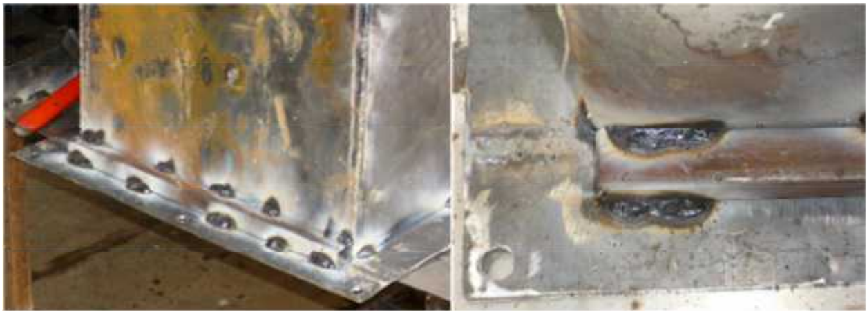
Picture 37: Square pipe attached to the back of the baking chamber flange (left), flush with top and bottom (right)
